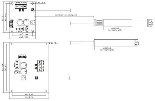
Fig. 1 Dimensions of EE1900
